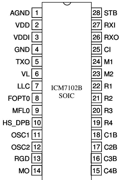
**Figure 1:** 28-lead SOIC Package
