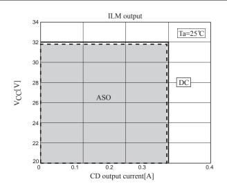
\*Characteristics of output current vs. output voltage (output pin).
