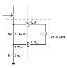
The ILM\_F voltage is determined by the internal band gap voltage of the IC (typ = 1.26V).
