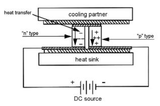
TEC1-00705T125 is a 1 stage, 7 couples, 2.8W peltierelement for cooling and heating
