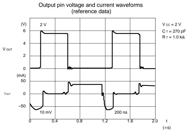
Note: The OFF delay time of  $V_{\text{OUT}}$  depends on the characteristics of the external transistor.
