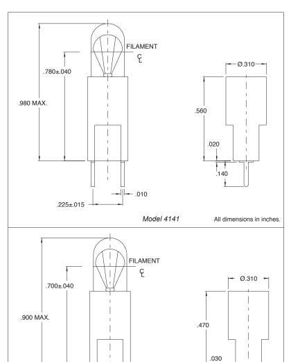
Mounting: Printed circuit Board
