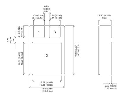
Bipolar NPN Device in a Hermetically sealed Ceramic Surface Mount Package for High Reliability Applications
