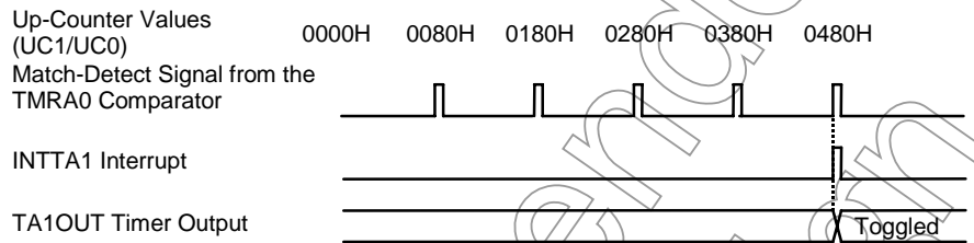
Figure 11.5 Timer Output in 16-Bit Interval Timer Mode
