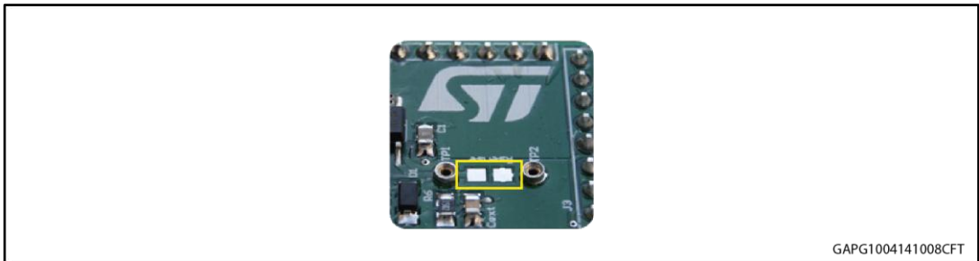
Figure 5: Pads for soldering SMD resistor
