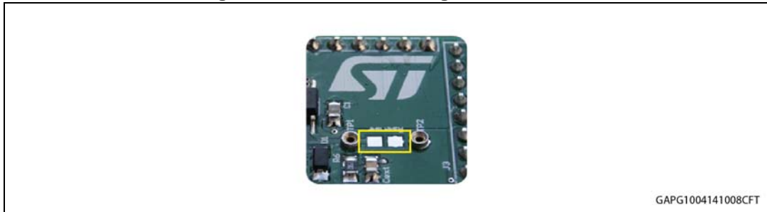
Figure 5. Pads for soldering SMD resistor
