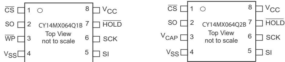
Figure 1. 8-pin SOIC pinout [1, 2]
