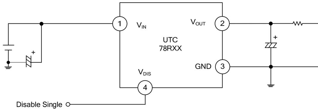
\*  $C_i$  is required if regulator is located an appreciable distance from power supply filter. [ $C_i > 0.33\mu\text{F}$  (Electrolytic)]
