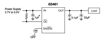
\*: 1µF of input capacitor is enough in most application cases.
