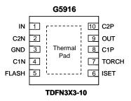
Note: Recommend connecting the Thermal Pad to the Ground for excellent power dissipation.
