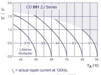
$I_R$  = rated ripple current at 120Hz, 85°C Multiplier of Useful Life as a function of ambient temperature and ripple current load
