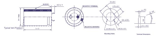
For diameter øD  $\ge$  45 mm the safety vent is typically placed at the side of the housing.
