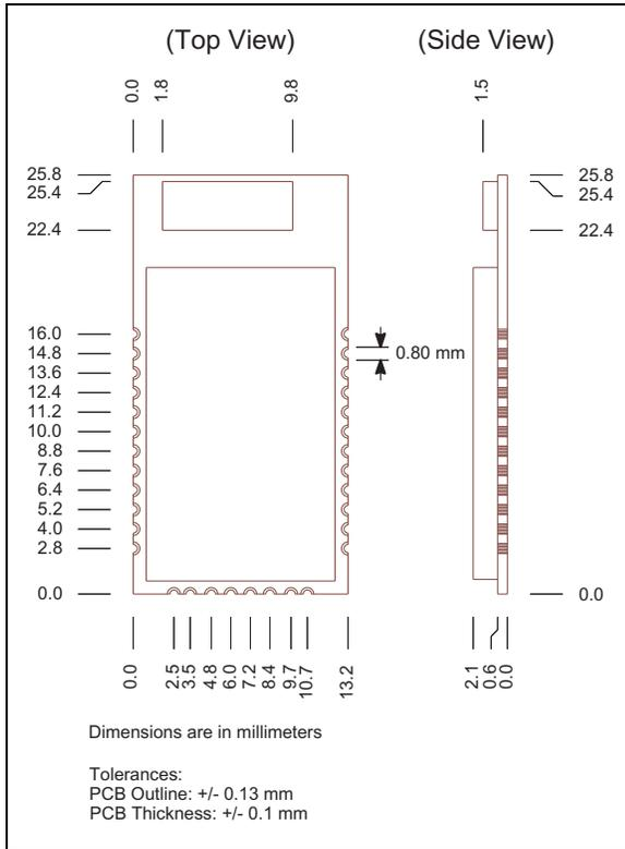
**FIGURE 1-3: RN41N MODULE DIMENSIONS**
