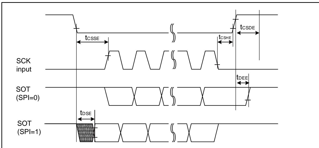
**When Using Synchronous Serial Chip Select (SPI = 1, SCINV = 0, MS=0, CSLVL=0)**
