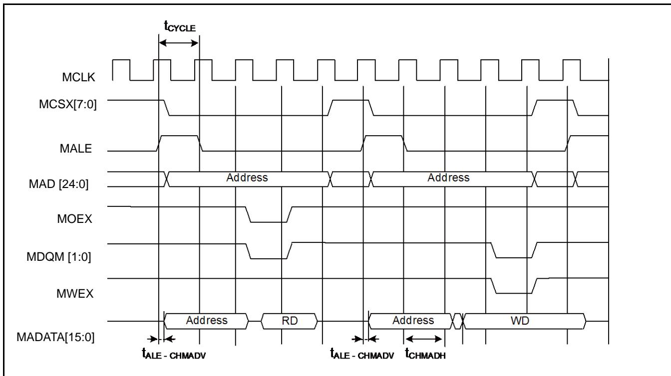
**Multiplexed Bus Access Synchronous SRAM Mode**
