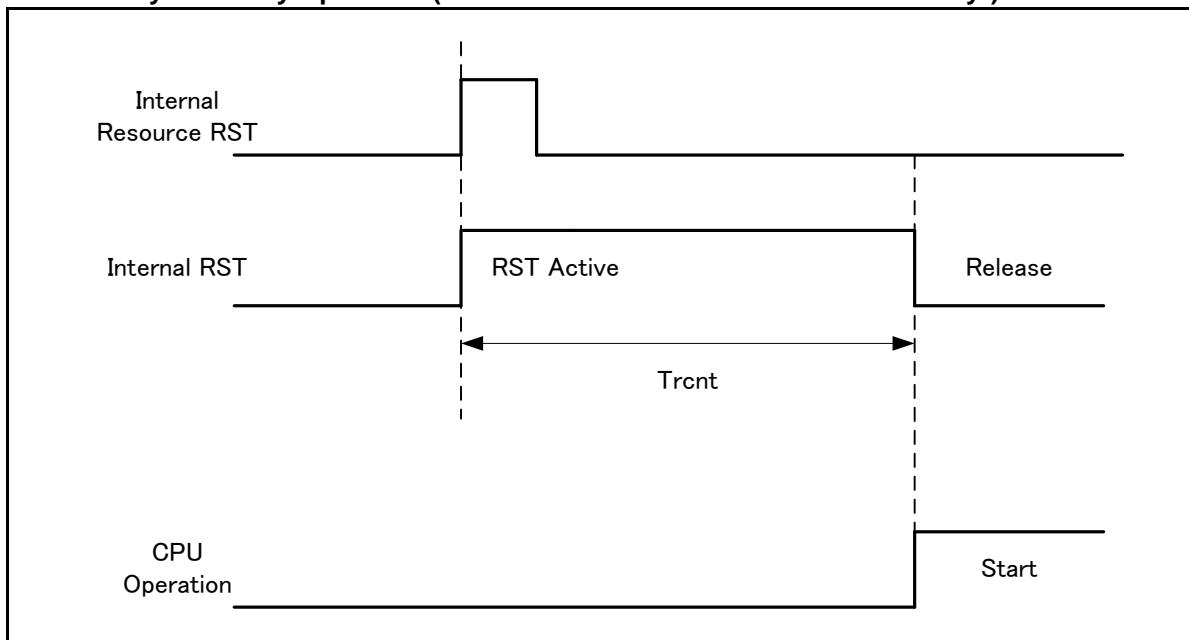
\*: Depending on the standby mode, the reset issue from the internal resource is not included in the recovery cause.
