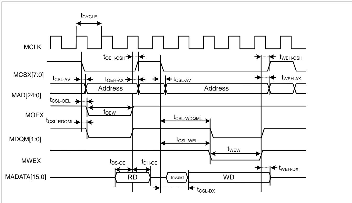
**Separate Bus Access Synchronous SRAM Mode**
