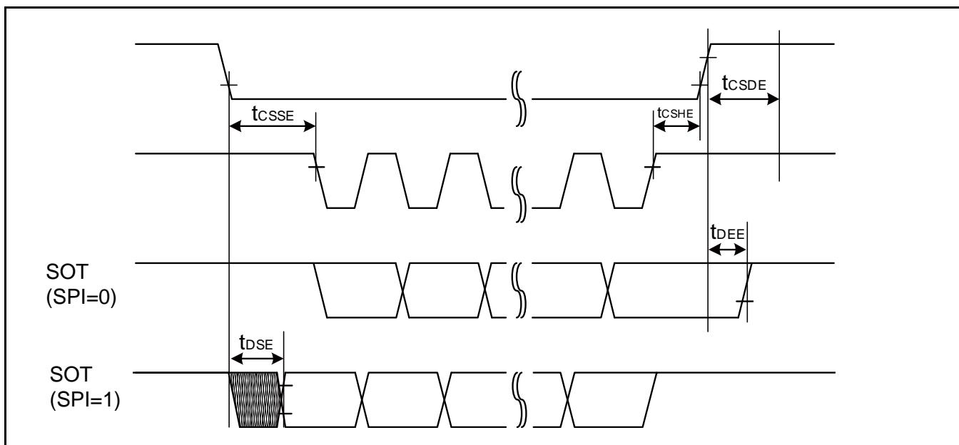
**When Using Synchronous Serial Chip Select (SPI = 1, SCINV = 1, MS=0, CSLVL=1)**
