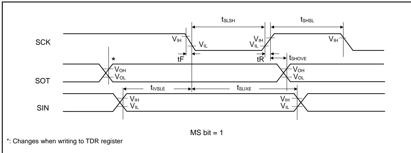
**High-speed Synchronous Serial (SPI = 1, SCINV = 1)**
