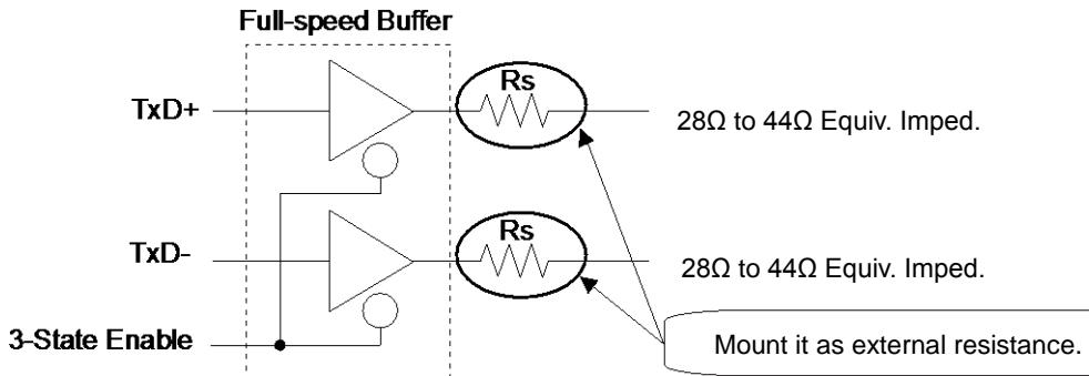
$R_s$  series resistor  $25\ \Omega$  to  $30\ \Omega$
