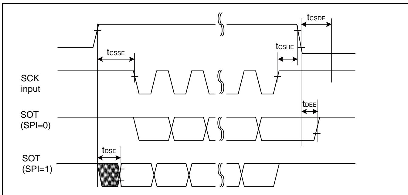
**When Using High-speed Synchronous Serial Chip Select (SPI = 1, SCINV = 1, MS=0, CSLVL=0)**
