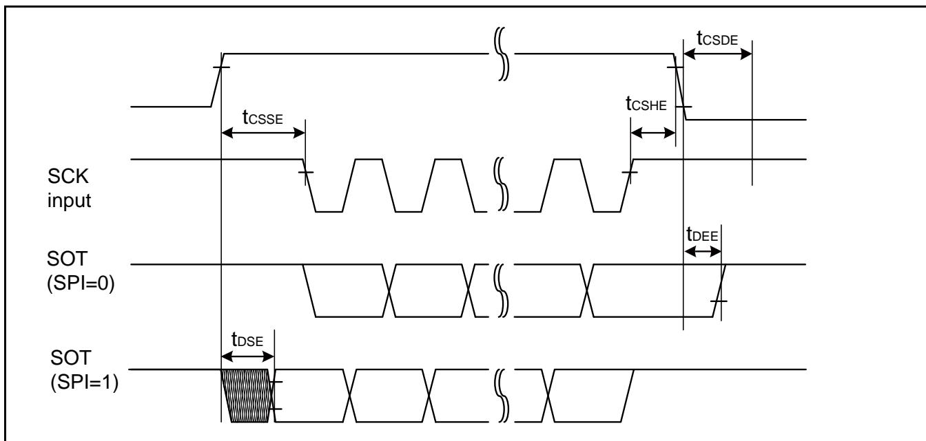
**When Using Synchronous Serial Chip Select (SPI = 1, SCINV = 1, MS=0, CSLVL=0)**
