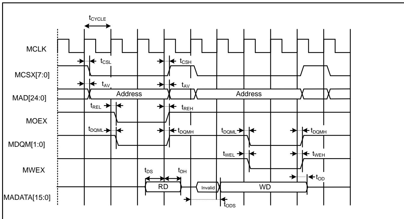
**Multiplexed Bus Access Asynchronous SRAM Mode**
