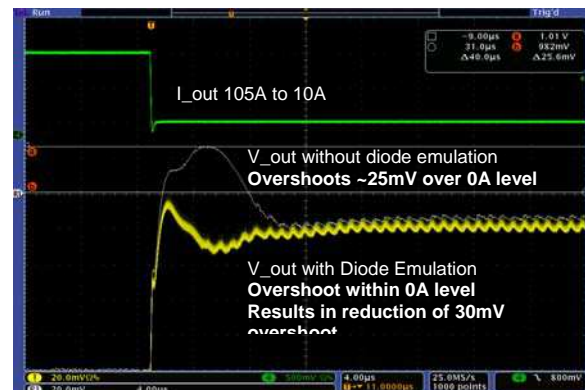
Figure 7: Output Voltage Overshoot Reduction with Diode Emulation
