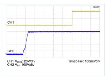
Figure 13 —  $V_{IN}$  to  $V_{OUT}$  start up wave form
