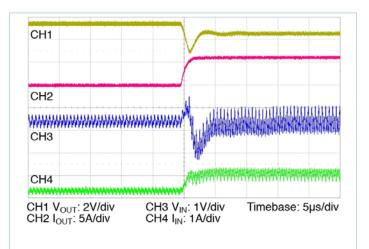
**Figure 15** — 0A - 7.7A transient response:  $C_{IN} = 330\mu F$ ,  $I_{IN}$  measured prior to  $C_{IN}$  no external  $C_{OUT}$
