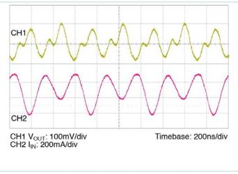
**Figure 14** — Output voltage and input current ripple;  $V_{IN} = 352V, 325W, \text{ no } C_{OUT}$
