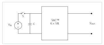
Figure 20 — Sine Amplitude Converter<sup>TM</sup> with input capacitor
