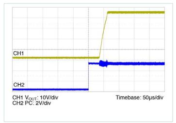
Figure 12 — PC to  $V_{OUT}$  start up wave form
