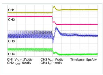
Figure 14 — 7.7A – 0A transient response:  $C_{IN} = 330\mu F$ ,  $I_{IN}$  measured prior to  $C_{IN}$  no external  $C_{OUT}$
