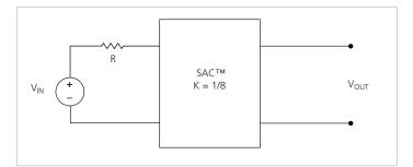
**Figure 19** — K = 1/8 Sine Amplitude Converter with series input resistor
