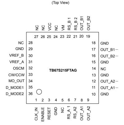
\* Please make sure to short the corner pads and the backside exposed pad to the ground pattern of the board.
