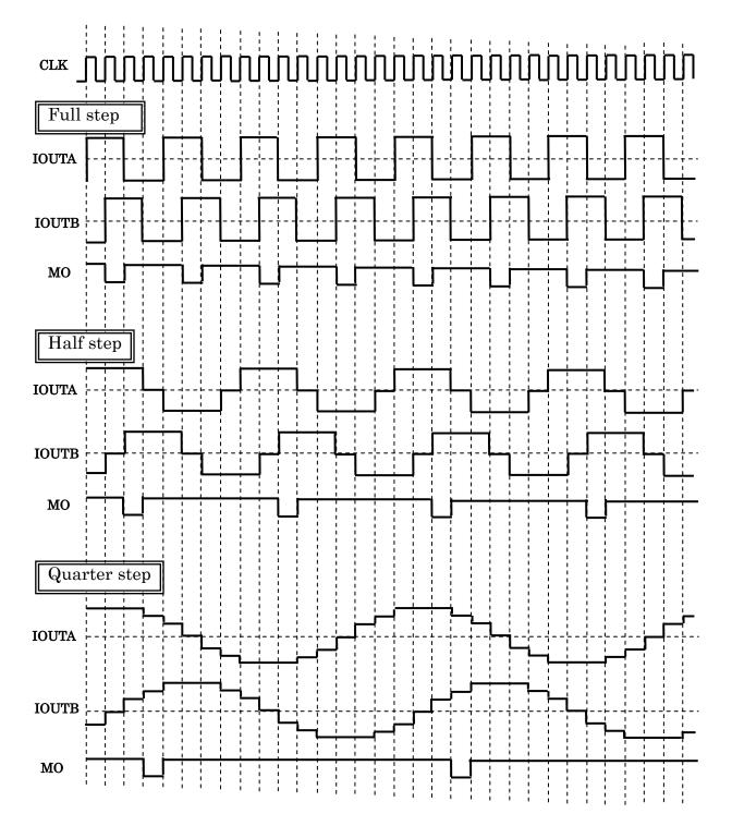
The MO is an open drain output pin. Therefore the High level of the MO waveform shown above, will be the MO pin's pulled up voltage level.
