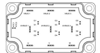
Pins NTC1 & NTC2 are only mounted on APTM100TA35SCTPG power module.
