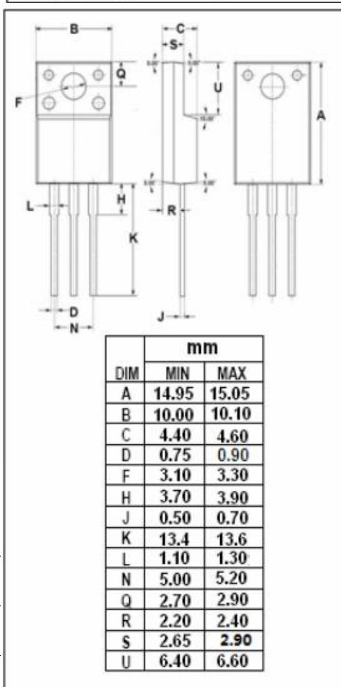
**Isc N-Channel MOSFET Transistor****TK30A06N1, ITK30A06N1****ELECTRICAL CHARACTERISTICS** $T_c=25^\circ\text{C}$  unless otherwise specified
