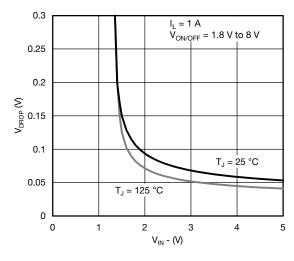
V<sub>DROP</sub> vs. V<sub>IN</sub> at I<sub>L</sub> = 1 A
