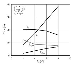
Switching Variation R2 at  $V_{IN}$  = 1.8 V, R1 = 20 k $\Omega$
