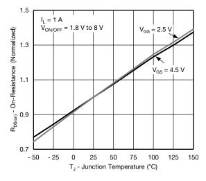
Normalized On-Resistance vs. Junction Temperature
