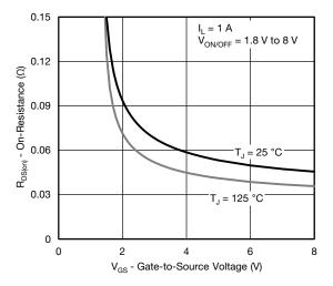
On-Resistance vs. Input Voltage
