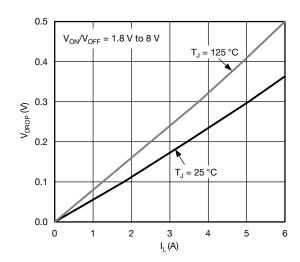
V<sub>DROP</sub> vs. I<sub>L</sub> at V<sub>IN</sub> = 1.8 V
