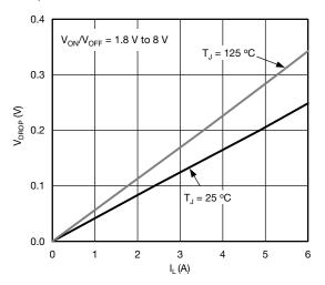
$V_{DROP}$  vs.  $I_L$  at  $V_{IN} = 4.5 \text{ V}$
