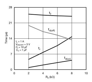
Switching Variation R2 at  $V_{IN}$  = 2.5 V, R1 = 20 k $\Omega$
