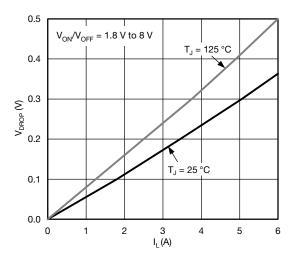
$V_{DROP}$  vs.  $I_L$  at  $V_{IN}$  = 2.5 V
