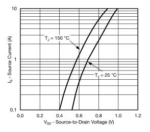
Source-Drain Diode Forward Voltage
