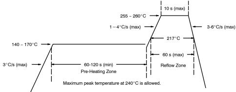
FIGURE 3. Solder Reflow Temperature and Time Durations
