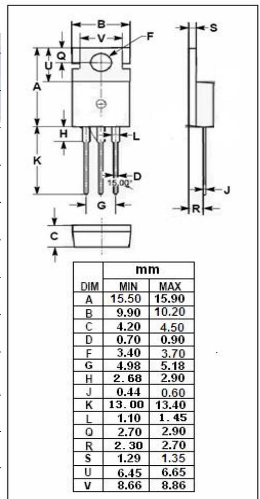
**isc N-Channel MOSFET Transistor**
