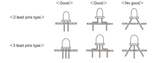
(2) Using spacer between LED's body and PCB is recommended. In case of direct mount on PCB(SLR/SLI-343 series), please take care about clinch of led pins to avoid the remained stress and solder heat stress. <u>Enough evaluation is requested before deciding assembly and soldering conditions.</u> <u>Please consult with us if any problems in the evaluation stage.</u>
